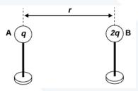
Sphere A exerts a force of magnitude F on sphere B. What is the magnitude of the force that sphere B exerts on sphere A?
