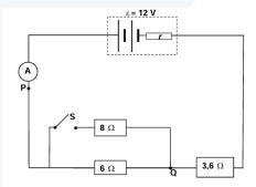
With switch S OPEN, ammeter A gives a reading of 1,2 A.
